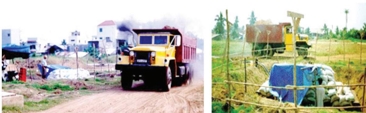
Fig 5. Site test for studying the additional settlement of model footing subjected to vibration
