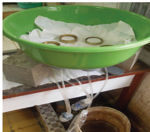
Figure 3. Modified leaching equipment
