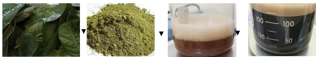
Figure 1. Schematic of synthesis of AgNPs by green synthesis method
