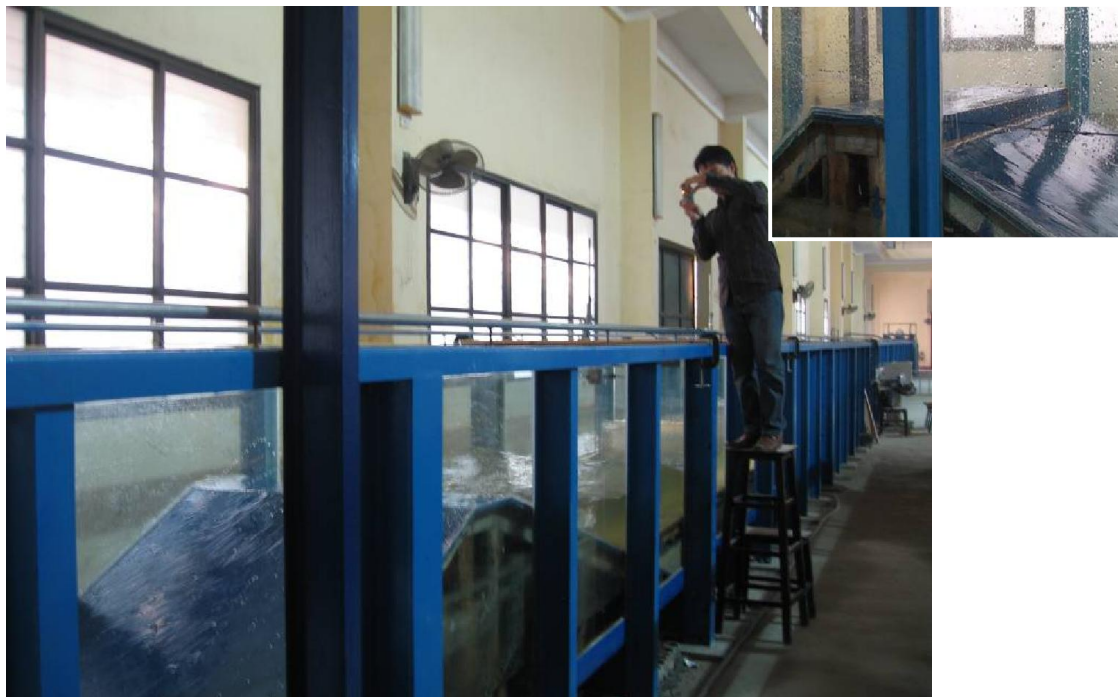
Figure 2. General layout of wave overtopping testing
