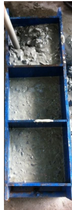
Figure 3. Fresh state performance of M7 (with chemical admixture)
