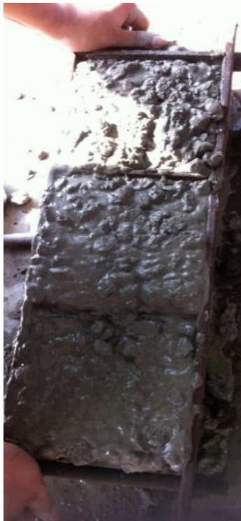
Figure 2. Fresh state performance of M5 (without chemical admixture)
