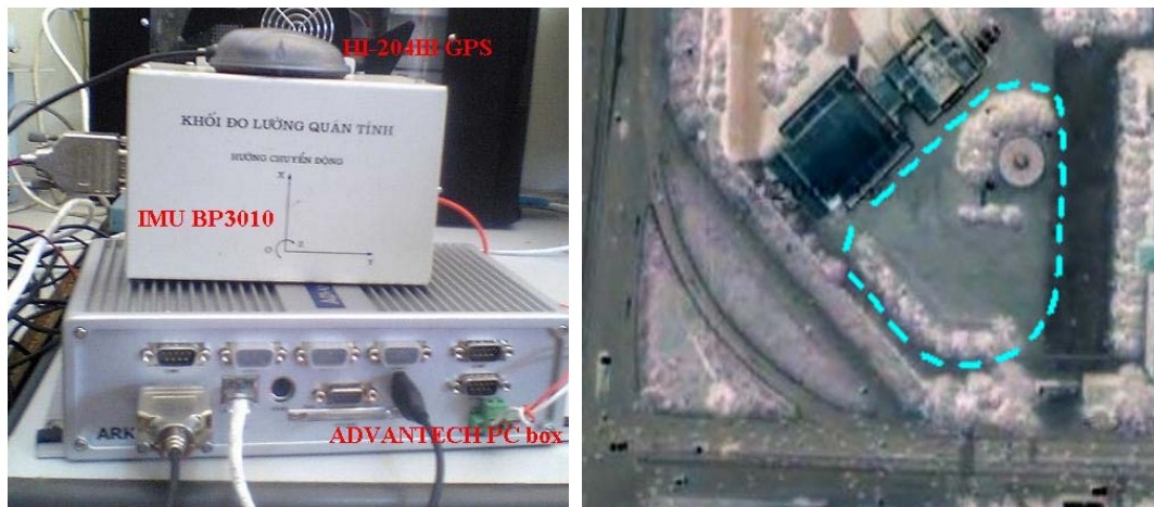
Fig 4. Hardware for the navigation system (a) and the trajectory of experimental vehicle (b)
