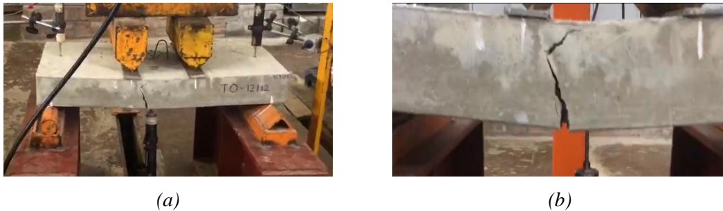
Fig. 7. Unreinforced slab: (a) under flexural failure and (b) failure mode.
