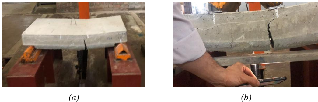
Fig. 8. TRC-strengthened reinforced concrete slabs: (a) under flexural failure and (b) failure mode.
