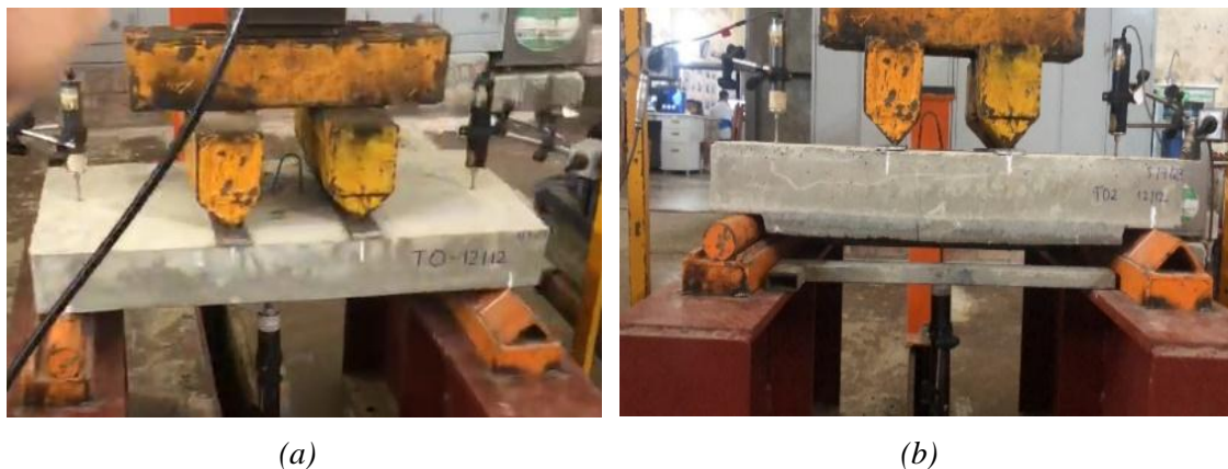
Fig. 6. Loading diagram for simply supported beam: (a) Unstrengthened reinforced concrete slab; (b) TRC-strengthened reinforced concrete slab.
