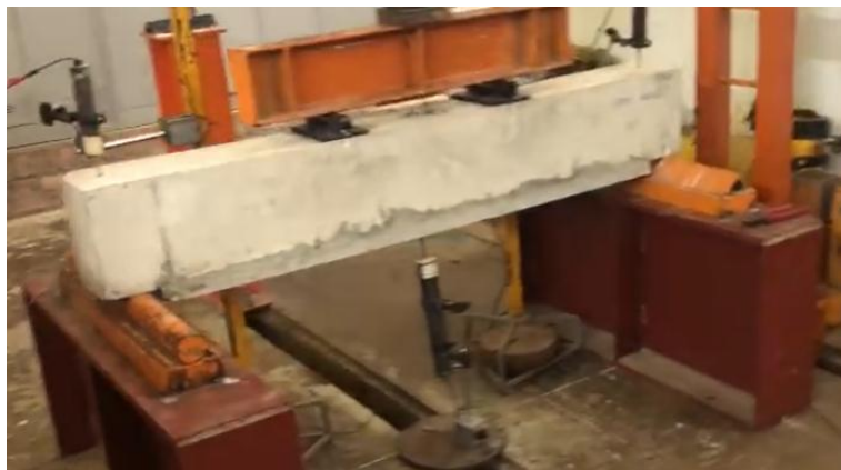
Fig. 7. Loading diagram for TRC reinforced simple beam.
