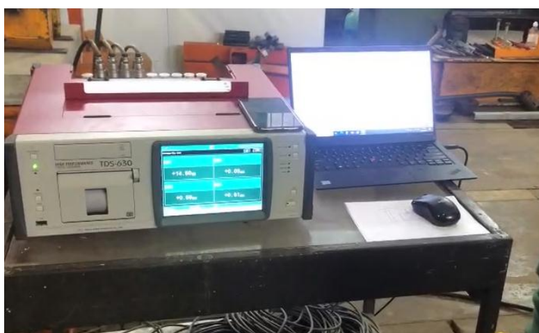
Fig. 8. Data logger TDS 530 combined with computer.
