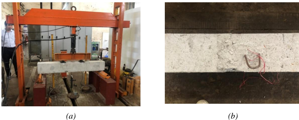
Fig. 9. Unstrengthened beam under bending: (a) before failure and (b) after failure.
