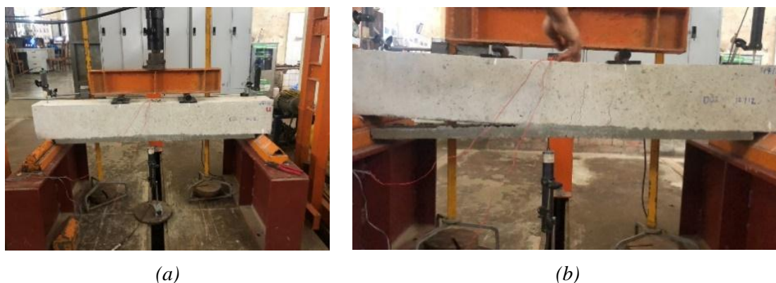
Fig. 10. Strengthened beam under bending: (a) before failure and (b) after failure.
