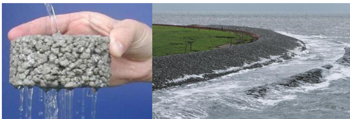
Fig. 3. Application of porous concrete in revetment.
