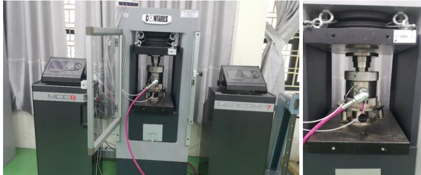
Figure 3.3. Automatic Triaxial test system MCC and Hoek cells
