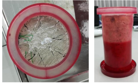
Figure 3.7. Failure in rock specimen
