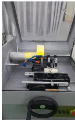
b) Core trimmer and cut-off machine
