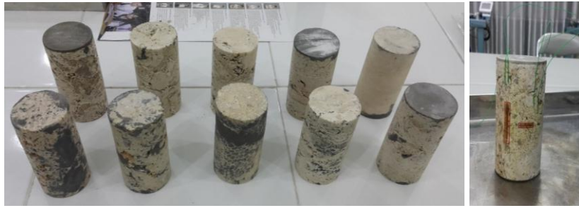
Figure 3.6. Coral rock specimens were 54×108mm in size
