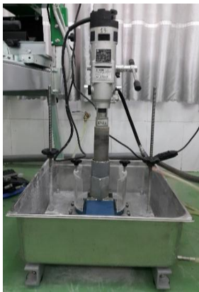
a) Laboratory coring machine and bits
