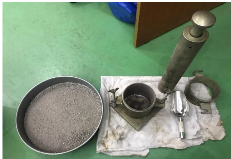
Figure 3. Testing devices for Proctor compacting tests
