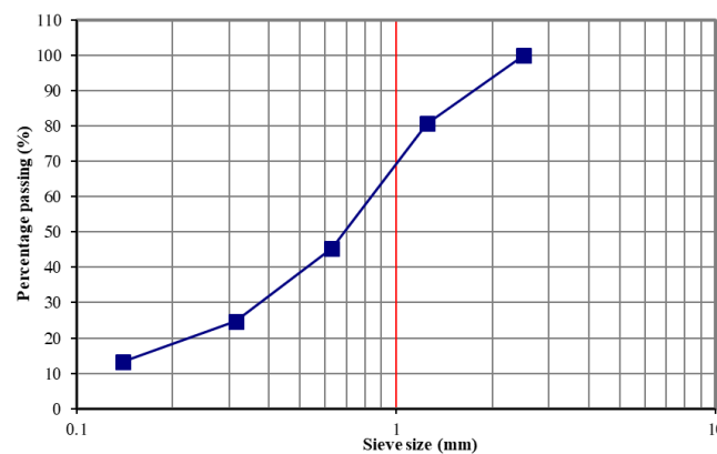
Figure 3. The grain-size distribution curve of the fine crushed stone.
