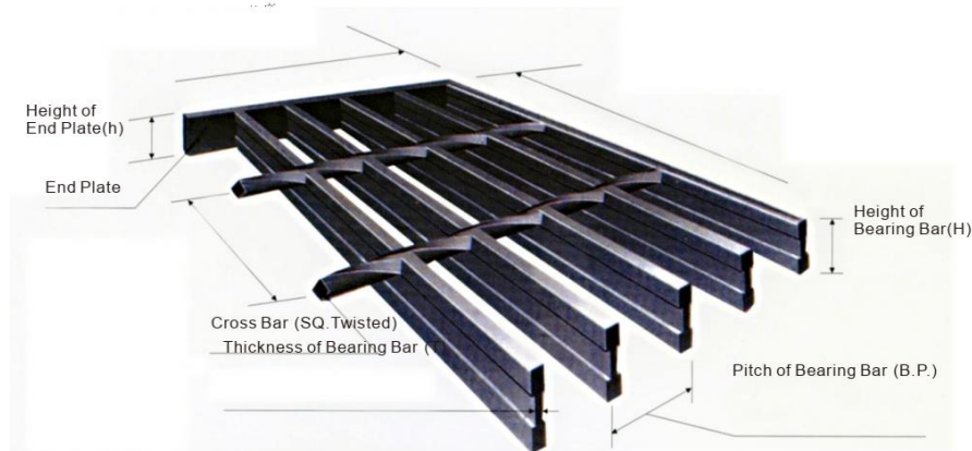
Figure 1. Structure of grating plate.
