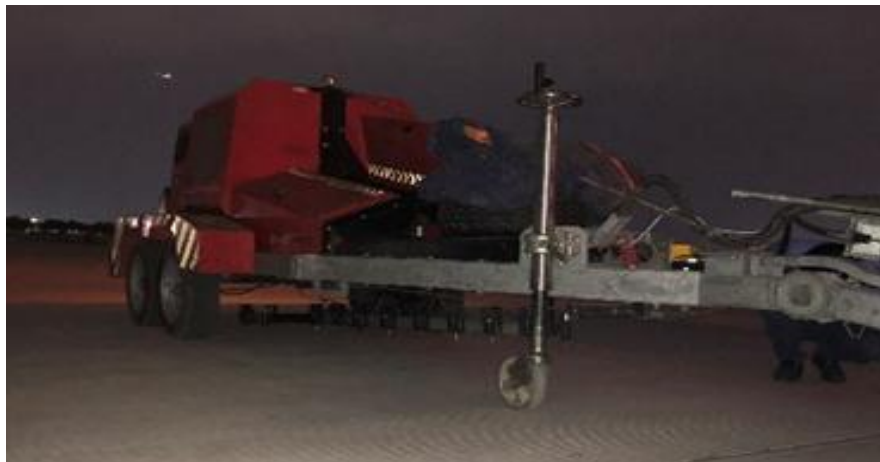
Fig. 5. Experimental measurement of road surface deflection.
