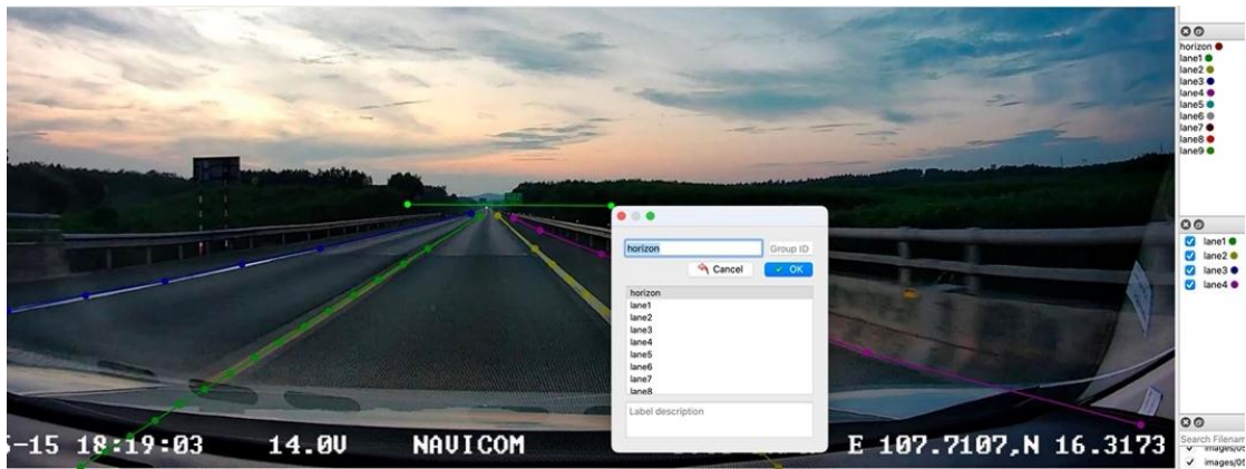
Fig. 4. Process of labeling the lanes (lane1, lane2, lane3, lane4) and vanishing-line (horizon).
