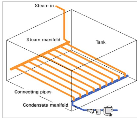
Figure 3: Steam Fuel Heating Diagram
