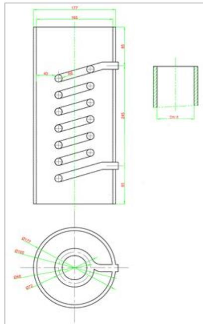
Figure 7: Structure of equipment utilizing exhaust heat
