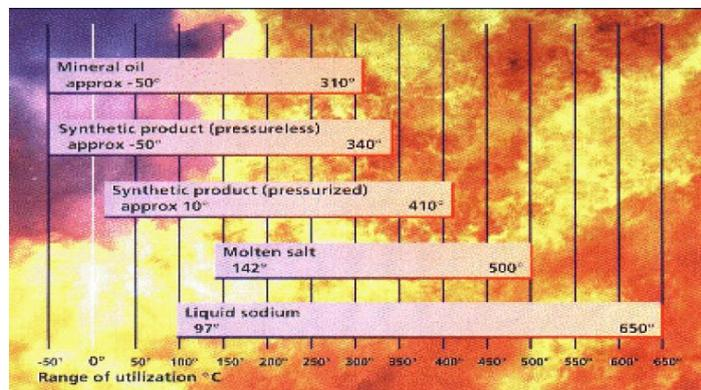
Figure 4: Operating temperature ranges of some thermal fluids
