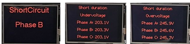
Fig. 9. The display screen indicates a short circuit fault and shows a warning of short-term under-voltage and over-voltage faults occurring in the electrical system
