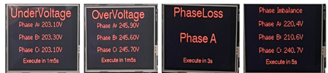
Fig. 10. The display screen shows the errors that have occurred in the electrical system along with the intervention time
