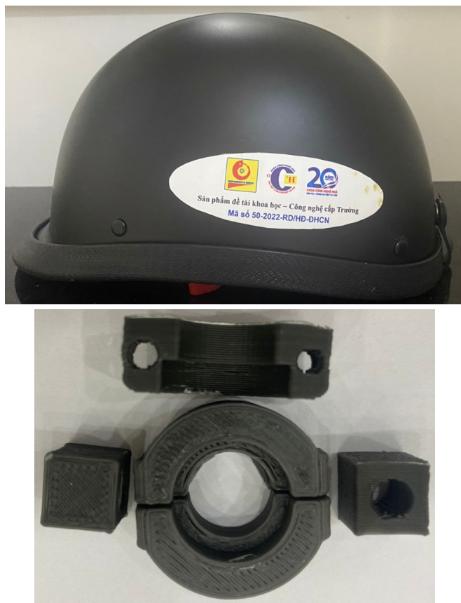
Figure 7. Helmet shell, clamp, nut made from PP/BCSi composite material
