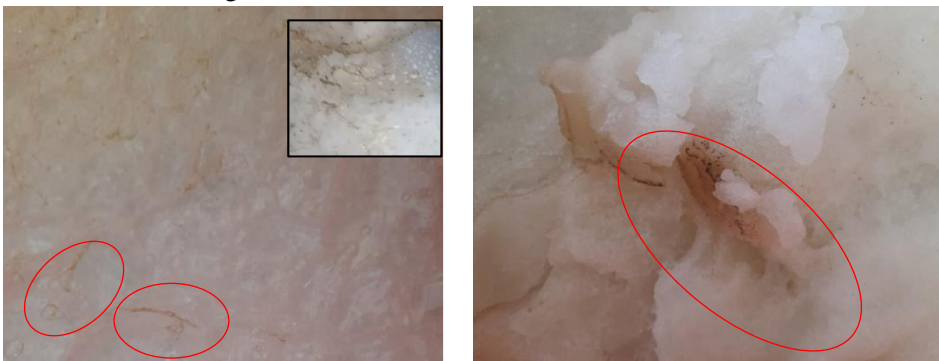
Figure 3. The picture of bubbles with impurities on surface of the tank
