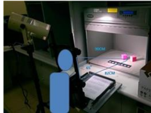
Figure 1. Viewing geometry for the grey scale method (diffuse and spot lighting)
