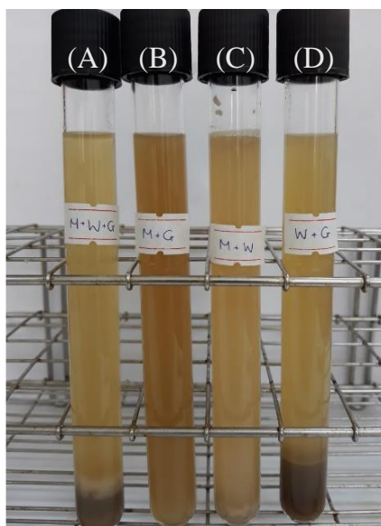
Figure 1. Sedimentation treatments of shell formulae (A) GA:WP:MD, (B) GA:MD, (C) WP:MD, and (D) GA:WP left at room temperature for 30 min
