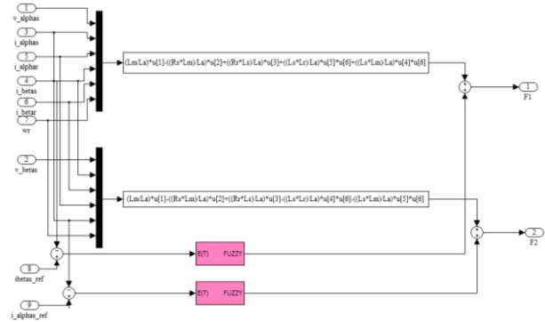
Figure 5. Fuzzy logic control signal generation block
