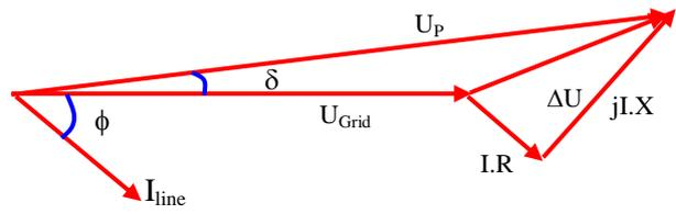
Fig. 5 Voltage Phasor Diagram
