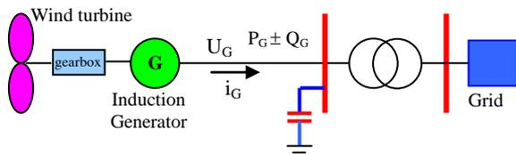
Fig. 1 Modelling wind turbine connected grid [1]
