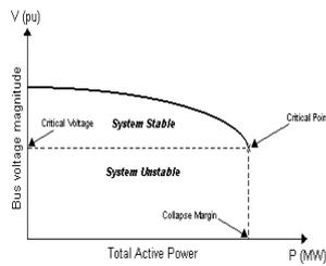
Fig. 2 Typical PU curve
