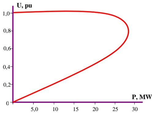
Fig. 12 PU curve at  $\phi = 20^\circ$  lead
