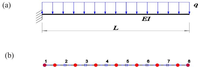
Figure 2b illustrates quadratic elements with each DOF per each control point (in circle). The displacement of the cantilever beam is plotted in Figure 3. As seen, the obtained result is in very
