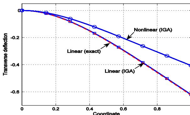
Figure 4 shows the variation of the deflection  $w$  at the free end of beam according to level of load. It can be recognized that the geometrically nonlinear results produce a stiffer reaction of the beam compared with the linear results. The stiffer behavior is explained by the additionally induced membrane stresses near the clamping point, which cannot be predicted by any linear theory.
