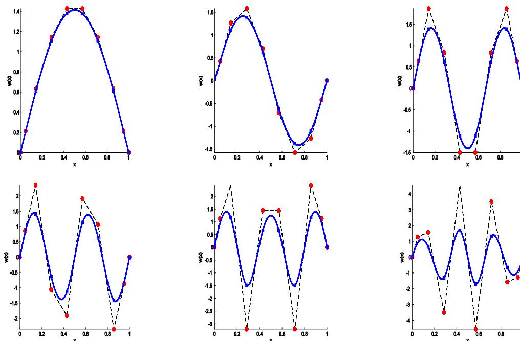
Now, let us consider a harmonic force excitation  $P = \sin(20t)$  applied at the middle of the beam. This problem is solved using the Newmark method (Chopra, 2007) with time step  $\Delta t = 10^{-3}$  s. Figure 8 reveals
