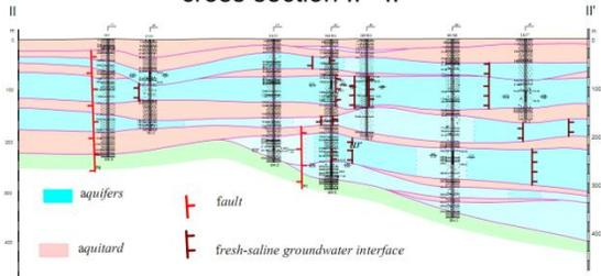
Figure 4. Hydrogeological cross-section II-II
