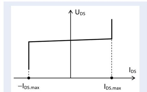
Figure 2: V-I characteristic of a STATCOM
