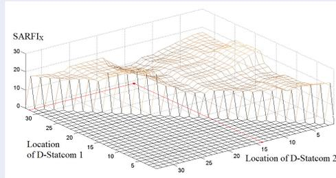
Figure 9: SARFI<sub>X</sub> for X=80% and I<sub>DSmax</sub> = 0.1p.u. as the function of all scenarios of 2 D-Statcom placement.
