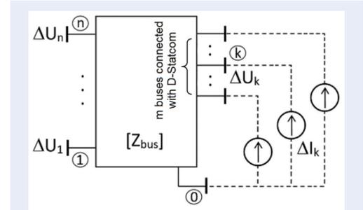
Figure 3: Test system short-circuit modeling using  $[Z_{bus}]$  with presence of m D-Statcoms ( $m < n$ ).
