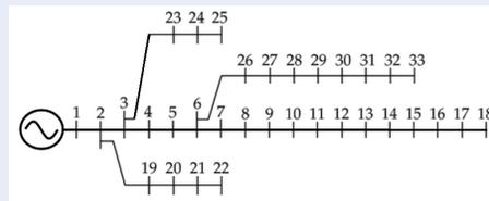
**Figure 7: IEEE 33-bus distribution feeder as the test system.**
