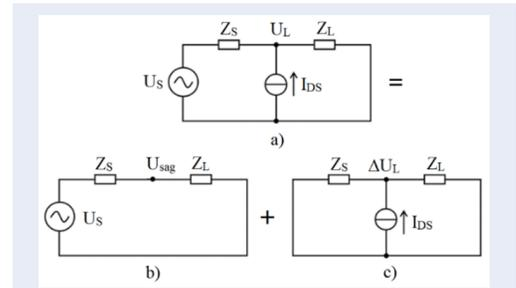
Figure 1: Modeling D-Statcom for voltage sag mitigation.
