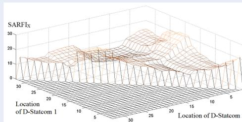
Figure 11: SARFI<sub>X</sub> for X=80% and I<sub>DSmax</sub> = 0.3p.u. as the function of all scenarios of 2 D-Statcom placement.
