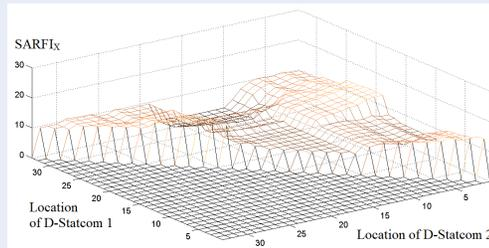
Figure 10: SARFI<sub>X</sub> for X=50% and I<sub>DSmax</sub> = 0.1p.u. as the function of all scenarios of 2 D-Statcom placement.
