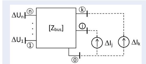
Figure 4: Test system short-circuit modeling using  $[Z_{bus}]$  with presence of two D-Statcoms.
