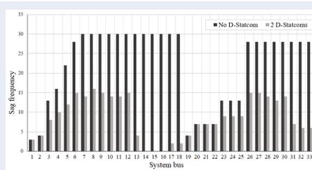
**Figure 8: Sag frequency for X=80% at system buses without and with two D-Statcoms,  $I_{DSmax} = 0.1p.u.$**
