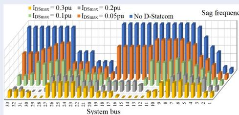
Figure 12: Sag frequency for X=80% at system buses without and with of two D-Statcoms (at optimal placement), for cases of I<sub>DSmax</sub> = 0.05, 0.1, 0.2, 0.3p.u.
