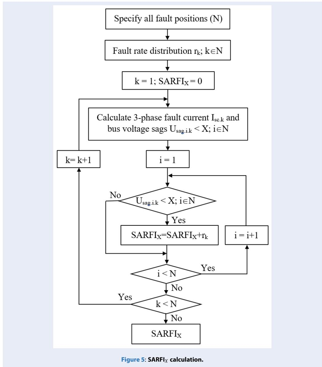
Figure 5: SARFI<sub>X</sub> calculation.
