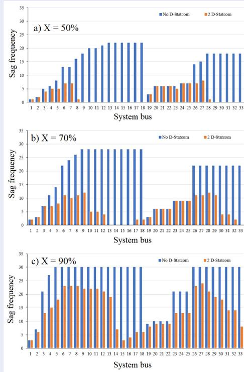
Figure 13: Sag frequency at system buses for X=50,70,90% without or with 2 D-Statcoms,  $I_{DSmax} = 0.1\text{p.u.}$  (at optimal placement).
