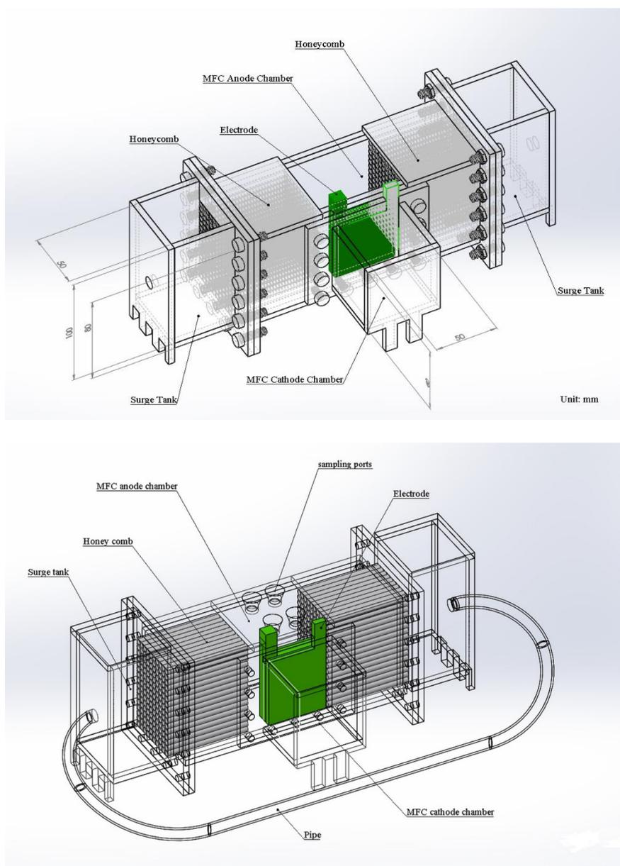
**Figure 2.** Perspective of two-chamber honeycomb MFC.<sup>36</sup>
