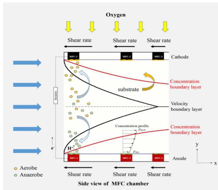
**Figure 3.** Diagram of boundary layers in a microbial fuel cell chamber.<sup>45</sup>
