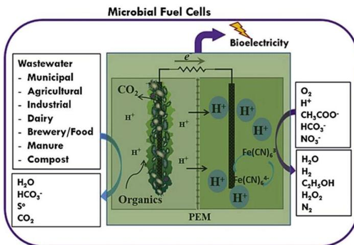
Figure 1. Structure diagram of microbial fuel cell.<sup>15</sup>
