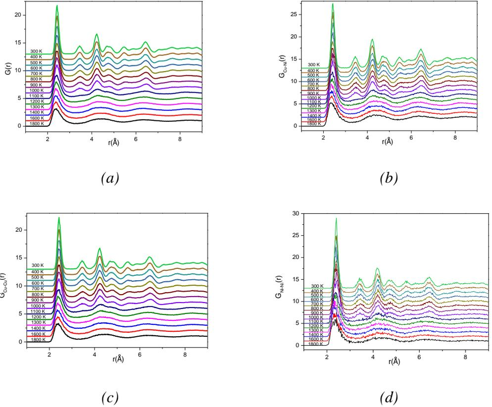
**Figure 3.** The RDF of  $\text{Cu}_{80}\text{Ni}_{20}$  samples at the pressure of 45GPa: a) The total radial distribution function  $G(r)$  of CuNi samples; b) The pair RDF  $G_{\text{Cu-Ni}}(r)$  for Cu-Ni pair; c) The pair RDF  $G_{\text{Cu-Cu}}(r)$  for Cu-Cu pair; d) The pair RDF  $G_{\text{Ni-Ni}}(r)$  for Ni-Ni pair
