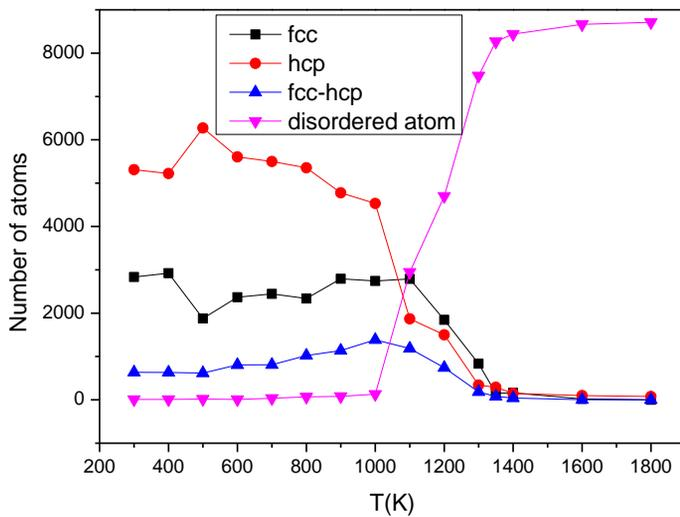
**Figure 2. Variations of FCC, HCP, HCP-FCC, and disordered atoms upon the cooling process at the pressure of 45GPa**
