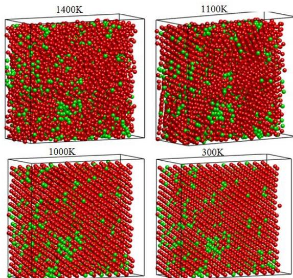
**Figure 5. Cross-sectional  $\text{Cu}_{80}\text{Ni}_{20}$  samples during the cooling process**
