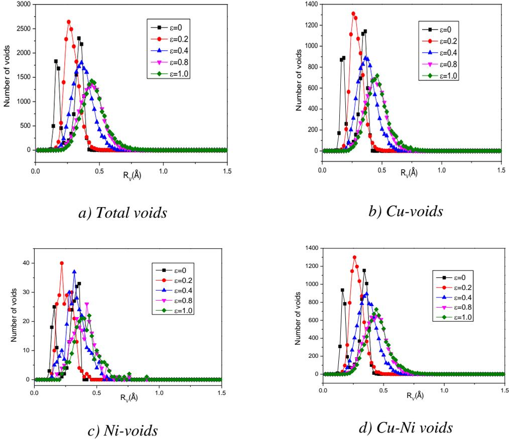
**Figure 8. The radii distributions of voids under uniaxial tension: a) Totals voids of the sample, b) Cu-voids, c) Ni-voids, and d) Cu-Ni-voids**
