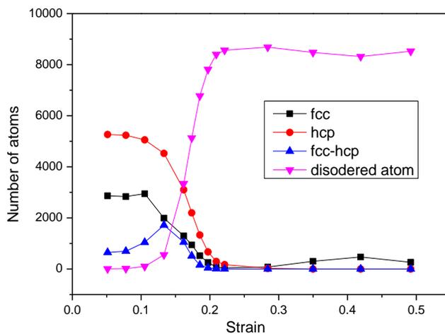
**Figure 7. The change of different kinds of atoms upon the uniaxial tension process at a pressure of 45 GPa**
