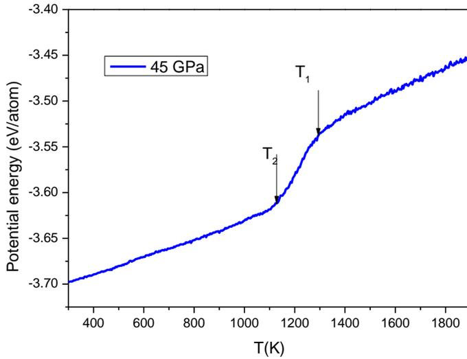
**Figure 1. Dependence on the temperature of potential energy under the cooling process at the pressure of 45 GPa**
