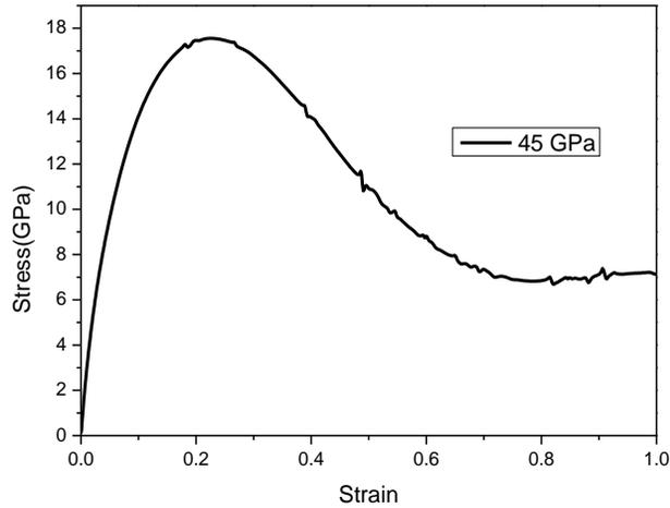
**Figure 6. The stress-strain curve of  $\text{Cu}_{80}\text{Ni}_{20}$  sample with the size of 8788 atoms at 300 K upon uniaxial tension**
