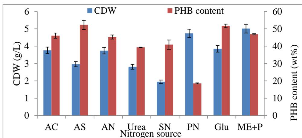
**Figure 3.** Effect of different nitrogen sources on the cell growth rate and PHB accumulation by strain *B. megaterium* D8
