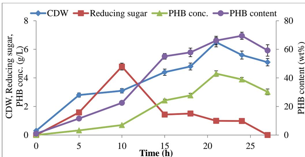
**Figure 4. Profile of the growth rate and PHB accumulation by strain D8 in a bioreactor using batch culture mode**
