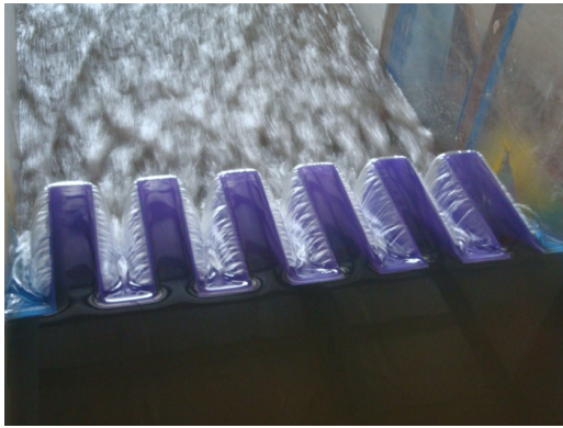
Figure 7. Flow over PKW in physical model
