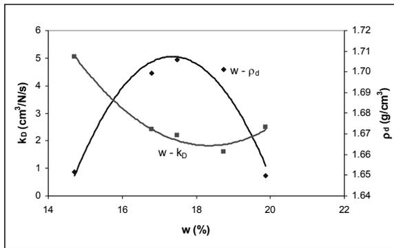
Figure 14: Relationship between the erosion coefficient,  $k_D$ , the dry density,  $\rho_d$  and the compaction water content,  $w$ , on the compaction curve
