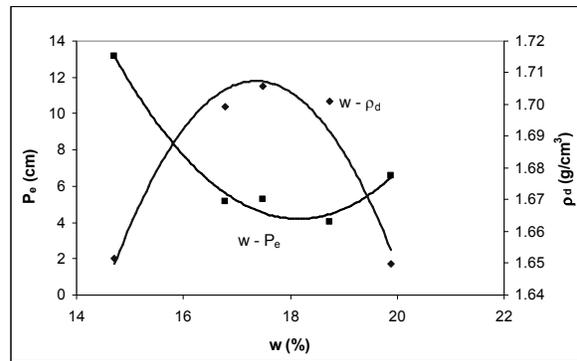
Figure 16: Relationship between the equilibrium erosion depth,  $P_e$ , the dry density,  $\rho_d$ , and the compaction water content,  $w$ , on the compaction curve
