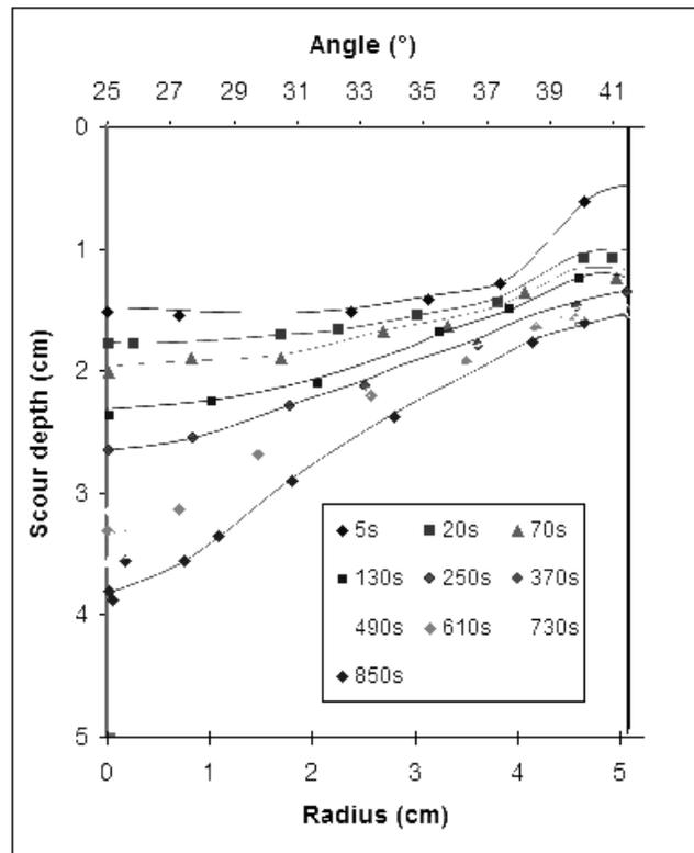
Figure 13: Example of erosion profiles corresponding to different measurement times
