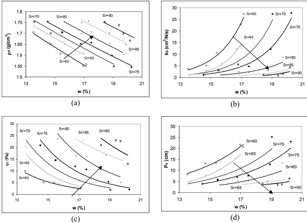
Figure 17: Relationship between the water content,  $w$ , the dry density,  $\rho_d$ , and the erosion parameters in the case of constant degree of saturation
