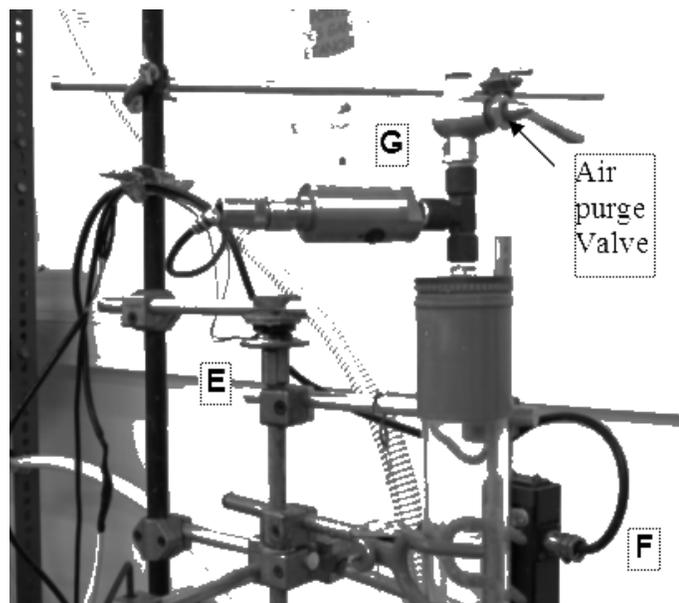
Figure 7: Pressure and angle sensors
