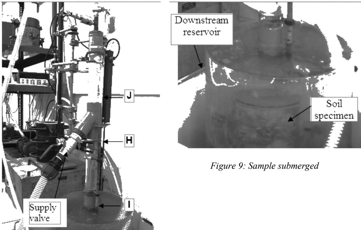
Figure 9: Sample submerged
