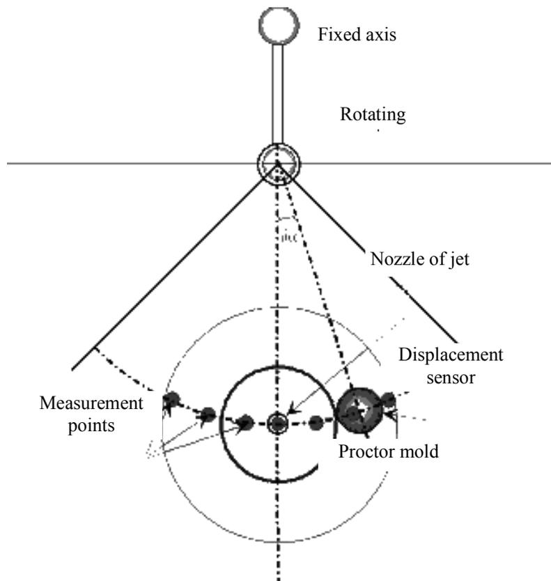
Figure 10: Displacement principle of the injection and measurement devices
