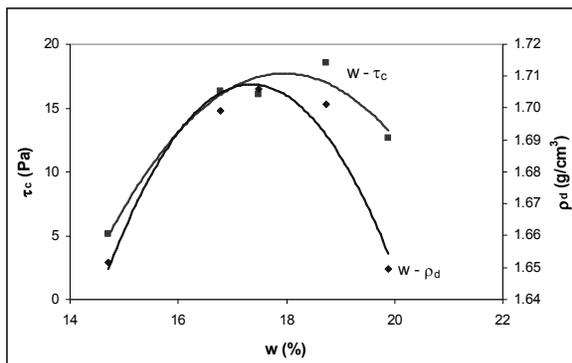
Figure 15: Relationship between the critical shear stress,  $\tau_c$ , the dry density,  $\rho_d$  and the compaction water content,  $w$ , on the compaction curve
