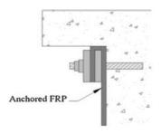
Figure 7. Schematic of typical U-Anchor
