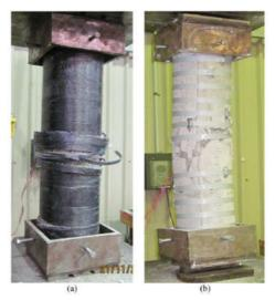
*Figure 11. Strengthening circular columns with (a) hoop FRP sheets, (b) steel strips*
