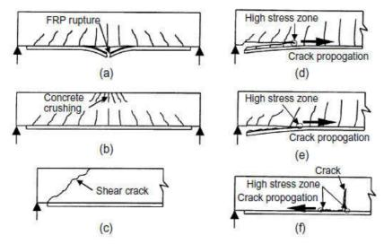
Figure 4. Failure modes of strengthened beams
