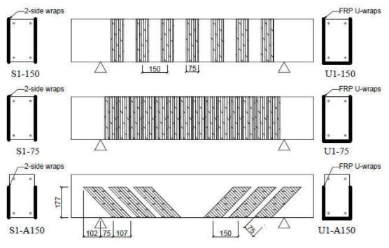
Figure 9. Strengthening beams in shear
