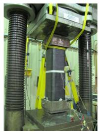
*Figure 10. Strengthening rectangular columns with hoop FRP sheets*
