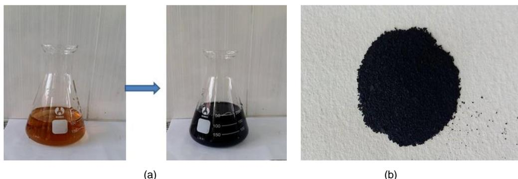
**Figure 1.** (a) The green tea extract turned to black when reacting with iron (II) solution; (b) ZVI nanoparticles
