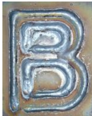
Fig 12. Heat effect on welding path
