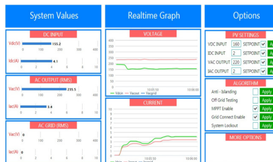
Figure 3. Web site monitor embedded in STM32F407
