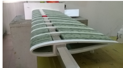
Figure 14. Preliminary wing models after assembled
