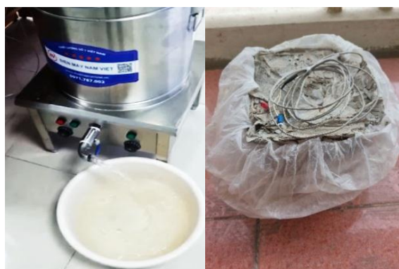
Fig. 10. Draining and removing sample from container.
