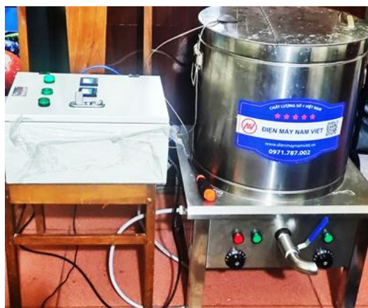
Fig. 9. Device for measuring adiabatic temperature.
