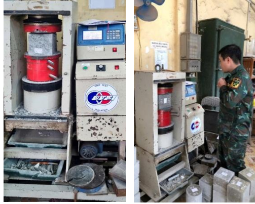
Fig. 4. Experiment to determine the compressive strength of concrete.
