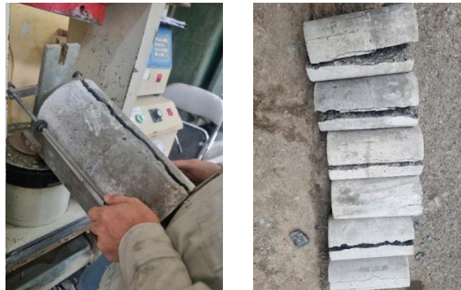
Fig. 5. Experiment to determine the tensile strength of concrete.
