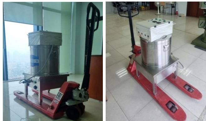
Fig. 7. Adiabatic temperature measuring device.
