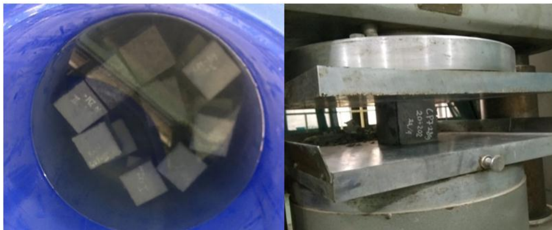
Figure 3. Test to determine compressive strength of concrete
