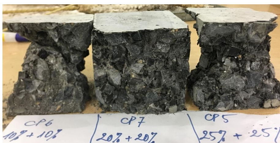
Figure 4. Test of compressive strength of concrete
