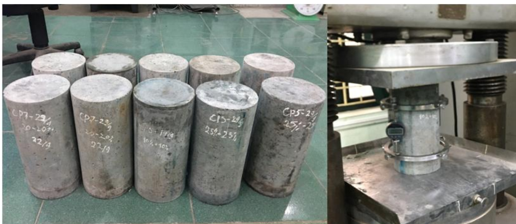
Figure 6. Test of static elastic modulus of concrete
