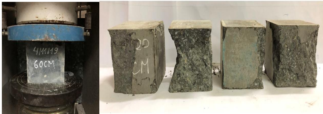
Figure 2. Failure pattern of the specimen subjected to compressive load.
