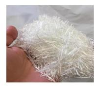
Figure 2. Reinforced glass fiber.
