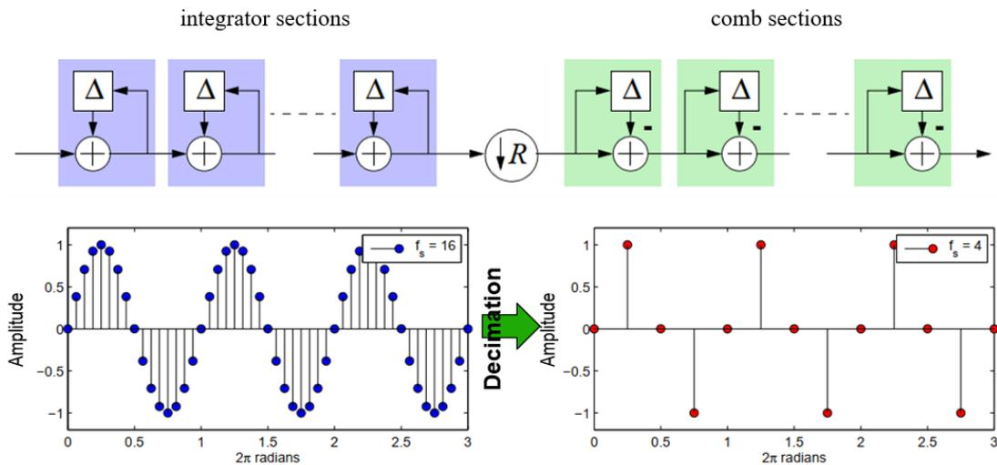
Fig. 4. Structure of the decimation CIC filter and its decimating processing
