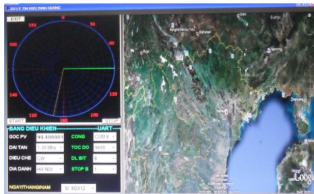
Fig. 10. DOA indicator at 90 degrees on computer.
