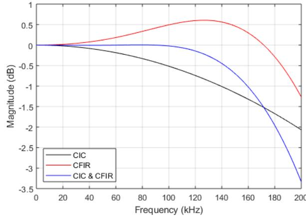
Fig. 5. Amplitude-frequency characteristic of the CIC, CFIR filters and their cascade
