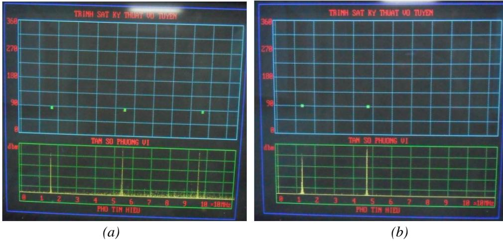
Fig. 9. Display results on VGA/LCD monitor: (a) when three signal frequencies are observed on the screen; (b) when two signal frequencies are observed on the screen.
