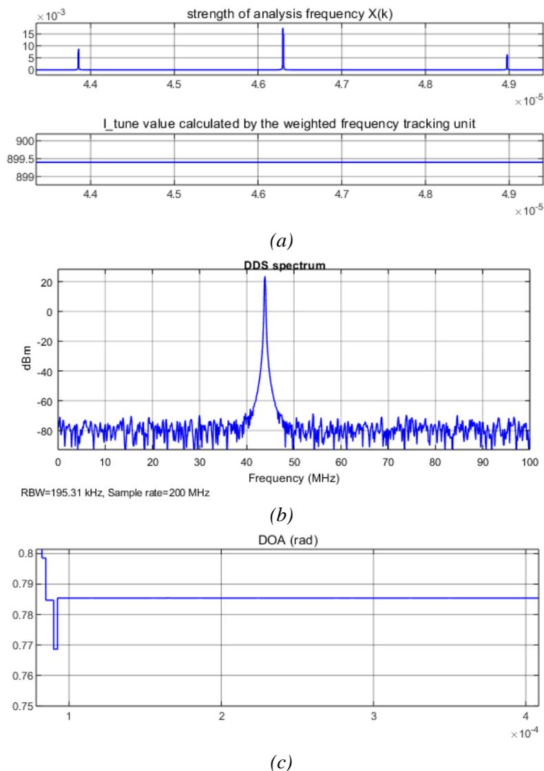
Fig. 7. Received results on System Generator for DSP tool: (a) Strength of the frequency components on the FFT output; (b) Signal generated by the DDS; (c) DOA estimation result.
