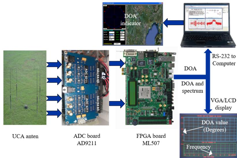
Fig. 8. Experimental setup of the proposed DOA estimation receiver
