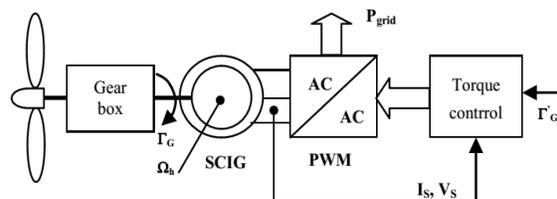
Figure 1. Diagram of the single wind turbine model
