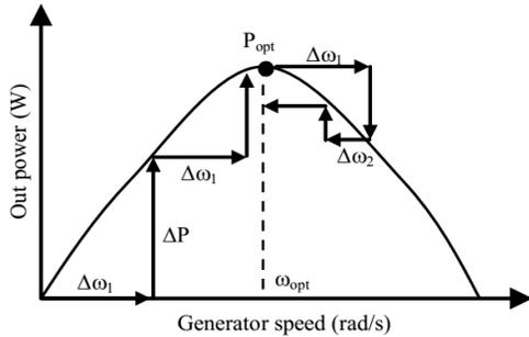
Figure 3. HCS technique for maximum power
