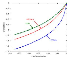
**Figure 4:** Nonlinear deflection of a CCCC PFGM plate made of Al/Al<sub>2</sub>O<sub>3</sub> with  $n = 3$ ,  $\xi = 0.3$ .
