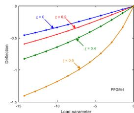
**Figure 3:** Nonlinear deflection of a SSSS PFGM-I plate made of Al/ZrO<sub>2</sub>-2 with  $n = 3$ .
