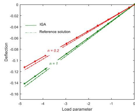
Figure 2: Nonlinear deflection of the PFGM plate made of Al/ZrO<sub>2</sub>-2
