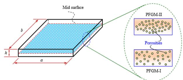
Figure 1: Geometry of FGM nanoplates with two porosity distributions.
