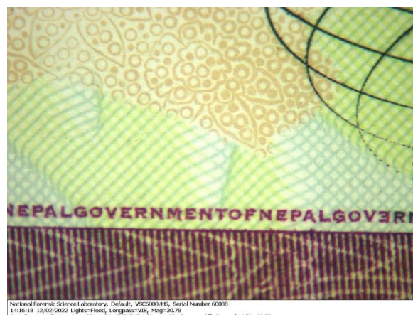
Figure 9: Micro-text present in Nepali passport under high magnification
