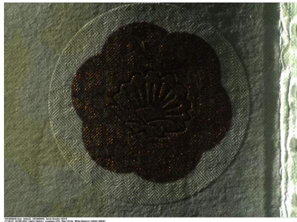
Figure 13: Emboss when viewed under high magnification and oblique light
