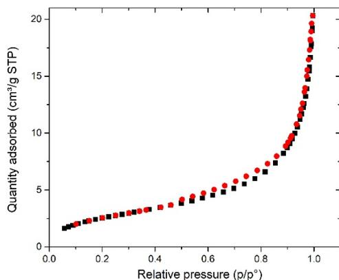
Figure 4. Nitrogen adsorption-desorption isotherms of ZnO nanoparticles
