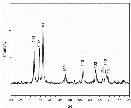
Figure 2: XRD patterns of ZnO particles
