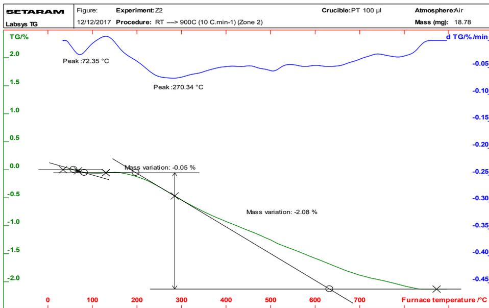
Figure 1. Thermo-gravimetric curves of ZnO nanoparticles
