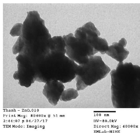
Figure 3: TEM image of the ZnO nanoparticles
