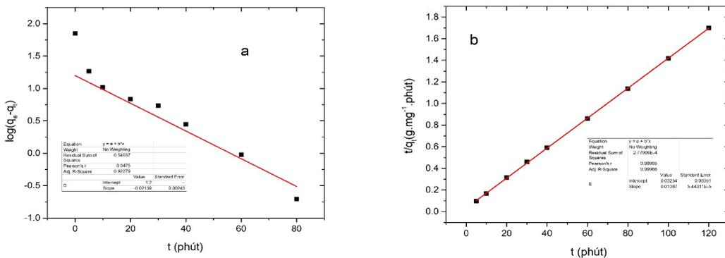
Figure 6: Pseudo-first-order kinetics (a) and pseudo-second-order kinetics (b) for congo red adsorption on the ZnO nanoparticles ( $T=30^{\circ}\text{C}$ , volume: 40 mL; adsorbent dose: 0.01 g; initial congo red concentration: 100 mg/L)
