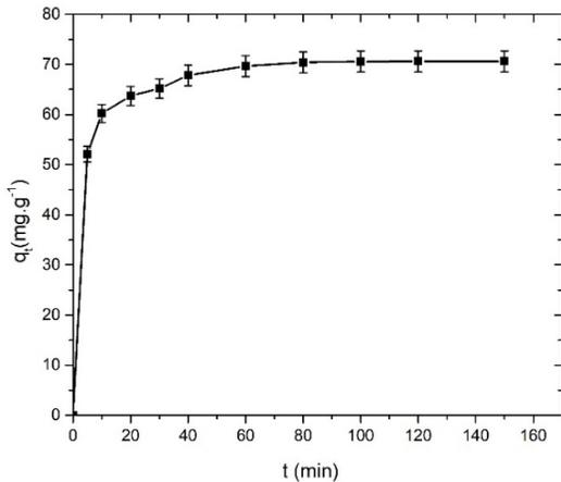
Figure 5. The relationship between adsorption capacity of congo red on ZnO nanoparticles and adsorption time ( $T=30^{\circ}\text{C}$ , volume: 40 mL; adsorbent dose: 0.01 g; initial congo red concentration: 100 mg/L)
