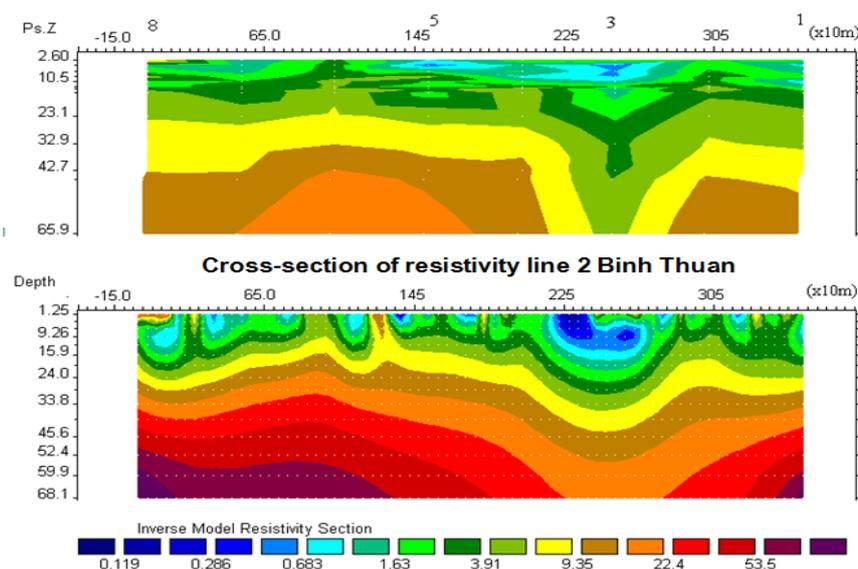
**Figure 2.** Resistivity section of line 2 Binh Thuan.
