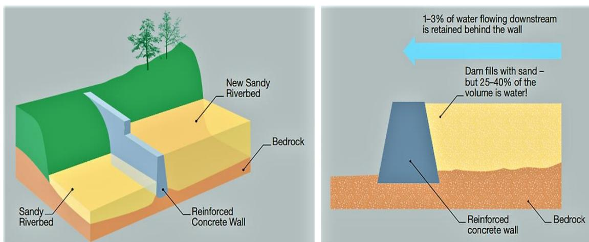
**Figure 11.** Left: Schematic cross-section of a sand dam. Right: Sand accumulates until the dam is completely full of sand up to the spillway. Water is stored within the sand, protected and filtered, making up to 40% of the total volume [19].
