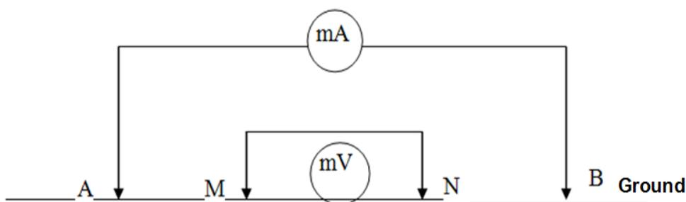
**Figure 4.** Diagram of method Schlumberger.
