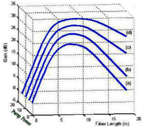
**Fig. 3.** Signal gain at 1550 nm as a function of EDF length for signal powers of  $P_{s1} = 1mW$ (a),  $P_{s2} = 2.5mW$ (b),  $P_{s3} = 0.125mW$ (c),  $P_{s4} = 0.06mW$ (d)
