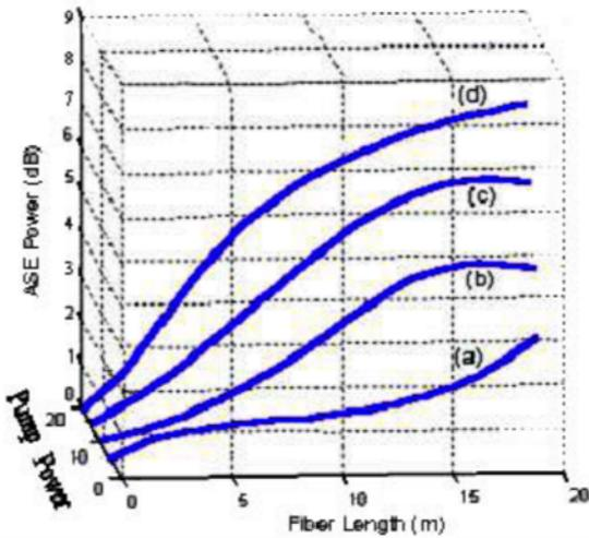
**Fig. 4.** ASE power as a function of EDF length for pump powers of  $P_{p1} = 10mW$ (a),  $P_{p2} = 20mW$  (b),  $P_{p3} = 30mW$  (c),  $P_{p4} = 40mW$  (d).
