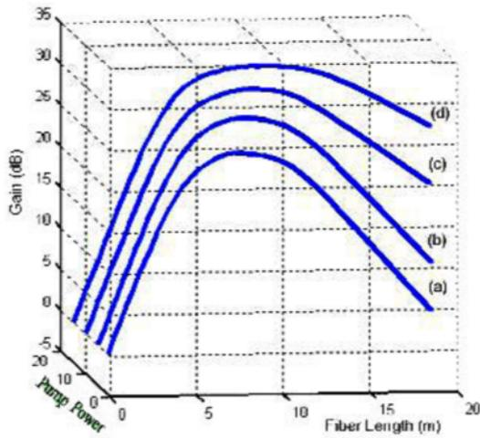
**Fig. 2.** Signal gain at 1550 nm as a function of EDF length for pump powers of  $P_{p1} = 10mW$ (a),  $P_{p2} = 20mW$  (b),  $P_{p3} = 30mW$  (c),  $P_{p4} = 40mW$  (d).
