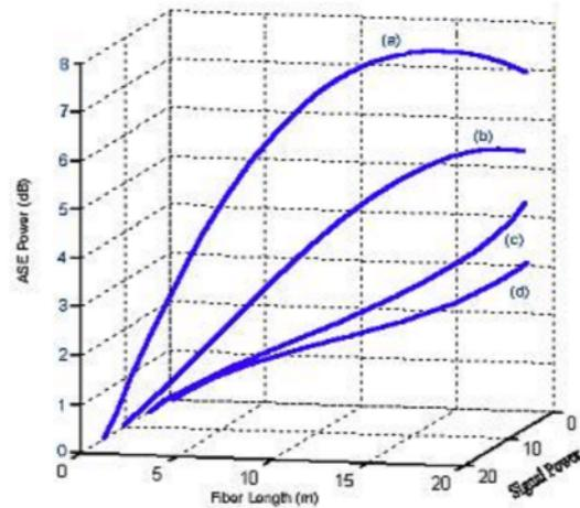
**Fig. 5.** ASE power as a function of EDF length for signal powers of  $P_{s1} = 1mW$ (a),  $P_{s2} = 2.5mW$ (b),  $P_{s3} = 0.125mW$ (c),  $P_{s4} = 0.06mW$ (d)
