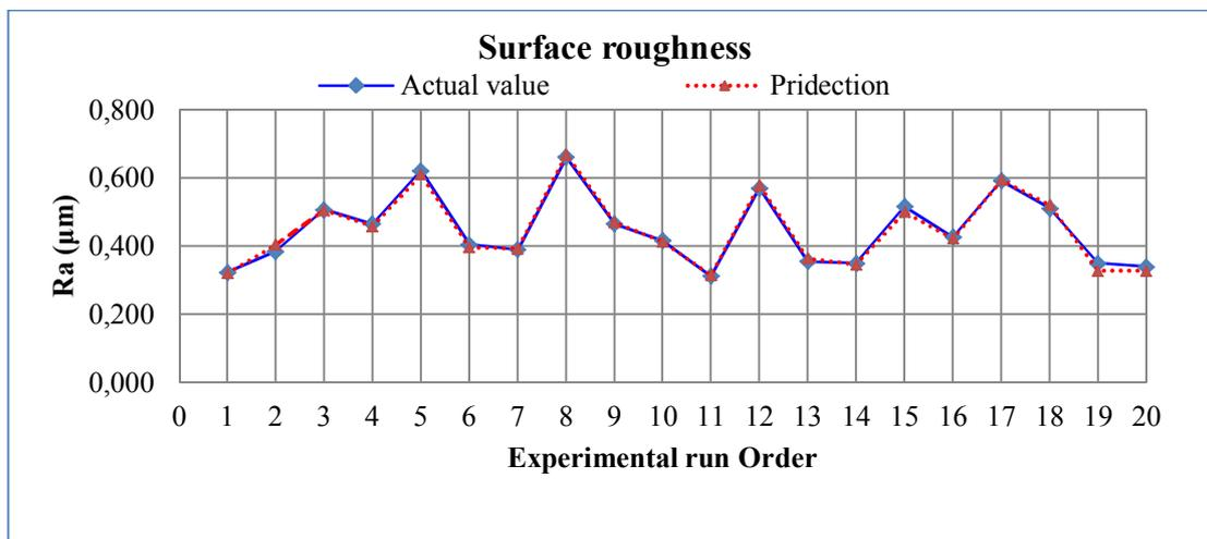
Fig. 3 Experimental and predicted values of surface roughness
