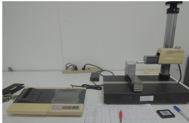
**Fig. 2.** Setting of surface roughness measurement
