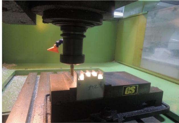
**Fig. 1.** Flank milling processes in a three-axis vertical machining Vcenter-4
