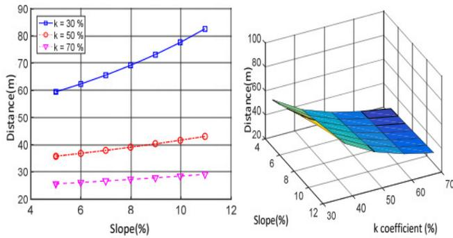
Figure 3. Investigation of braking distance with road gradients ranging from 5% to 11% and pedal brake travel ratio  $k$  varying from 30 to 70% (supplementary brake torque  $M_b = 20\text{Nm}$ ; adhesion coefficient  $\phi = 0.7$ ,  $v_1 = 60\text{km/h}$ ,  $v_2 = 20\text{km/h}$ ).
