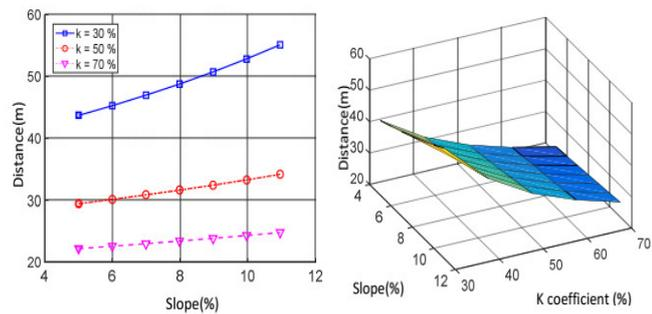
Figure 4. Investigation of braking distance with road gradients ranging from 5% to 11% and pedal brake travel ratio  $k$  varying from 30 to 70% (supplementary brake torque  $M_b = 80\text{Nm}$ ; adhesion coefficient  $\phi = 0.7$ ,  $v_1 = 60\text{km/h}$ ,  $v_2 = 20\text{km/h}$ ).
