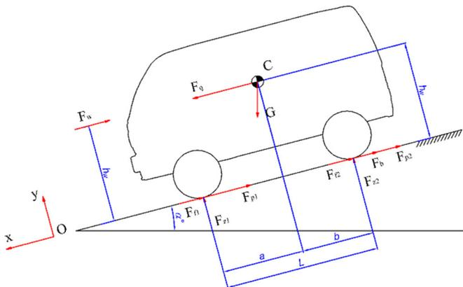
Figure 1. Forces and moments acting on van truck when descending a slope and braking
