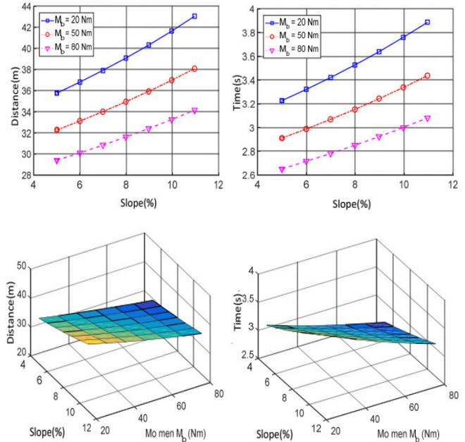
Figure 2. Investigation of braking distance and braking time with road gradients ranging from 5% to 11%, supplementary brake torque  $M_b$  varying from 20 to 80Nm (adhesion coefficient  $\varphi = 0.7$ ,  $v_1 = 60\text{km/h}$ ,  $v_2 = 20\text{km/h}$ , pedal brake travel ratio  $k = 50\%$ )
