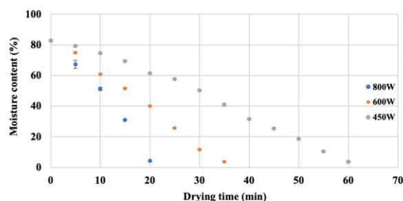
**Figure 1.** Drying curves of noni fruit at different microwave power levels
